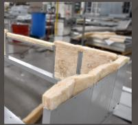
The unit casing is a double-break, formed panel design providing rigidity while encapsulating insulation. Optional thermal break design is available using a low-thermal conductive neoprene gasket between the interior and exterior metal surfaces to act as a barrier against thermal transmission and preventing sweating.
